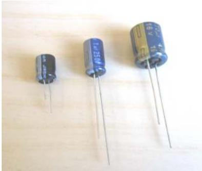
Figure 11: Electrolytic capacitors
