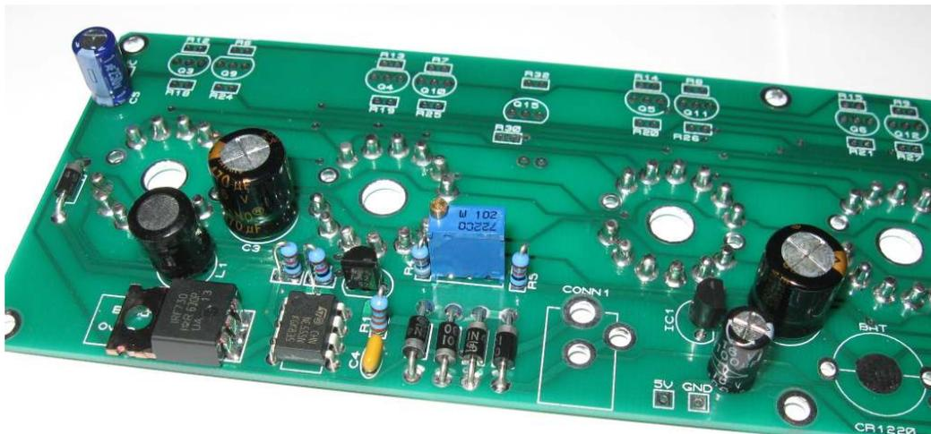
Figure 12: Electrolytic capacitors placed on the PCB
