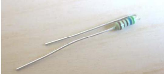
Figure 7: Resistor leads formed for mounting upright.
