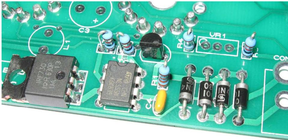
Figure 8: R1 to R5 placed vertically
