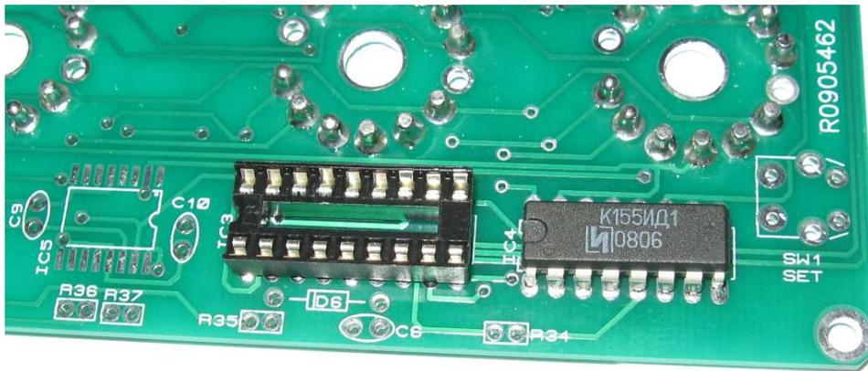
Figure 15: Socket for IC3, and IC4
