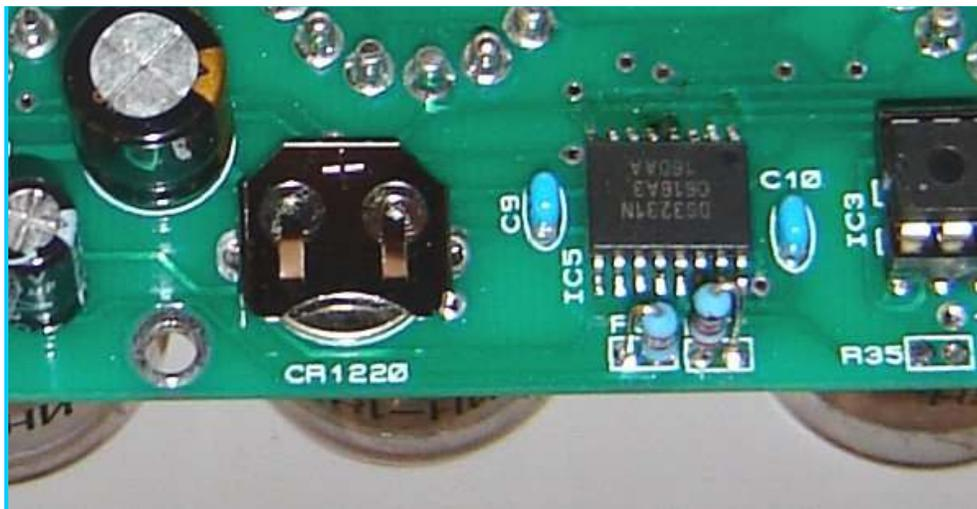
Figure 18: Showing all RTC components: IC5, C9, C10, R36, R37, Lithium Cell
