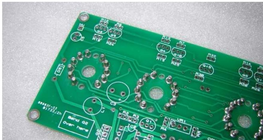
Figure 2: 1mm sockets placed noting 2 holes per tube without socket
