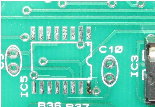
Figure 16: Corner SMD pad wetted with solder
